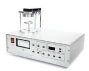
The automatic sputter coater deposits a fine gold layer onto samples using high-vacuum sputtering. Argon plasma ablates gold atoms from a target, depositing them evenly on the sample. Metallisation is essential to render biological samples conductive, reduce charging, and preserve ultrastructural detail during SEM analysis.
